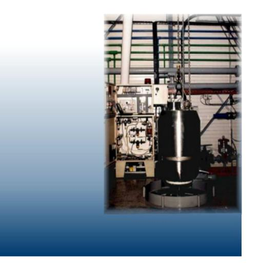
The rotary atomizer is a direct-drive, high-frequency, two-pole electrical motor designed for a VFD power supply in the range above 200Hz, thereby creating rotating wheel speeds in excess of 12.000 RPM. The atomizer is further supplied with an integral local control panel, and also may be controlled directly by plant's DCS. Dedicated atomizer software is supplied with the control system.
